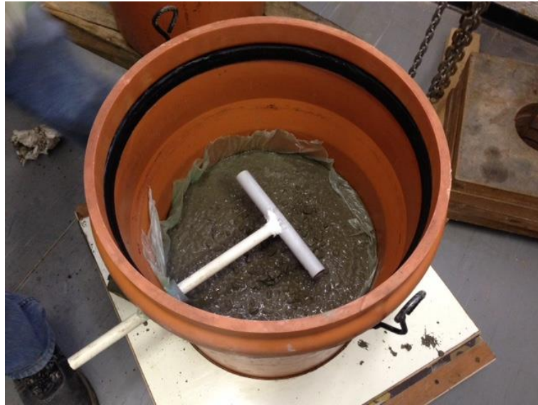
Figure 2: Concrete chamber before assembly into the pipe and air inlet
