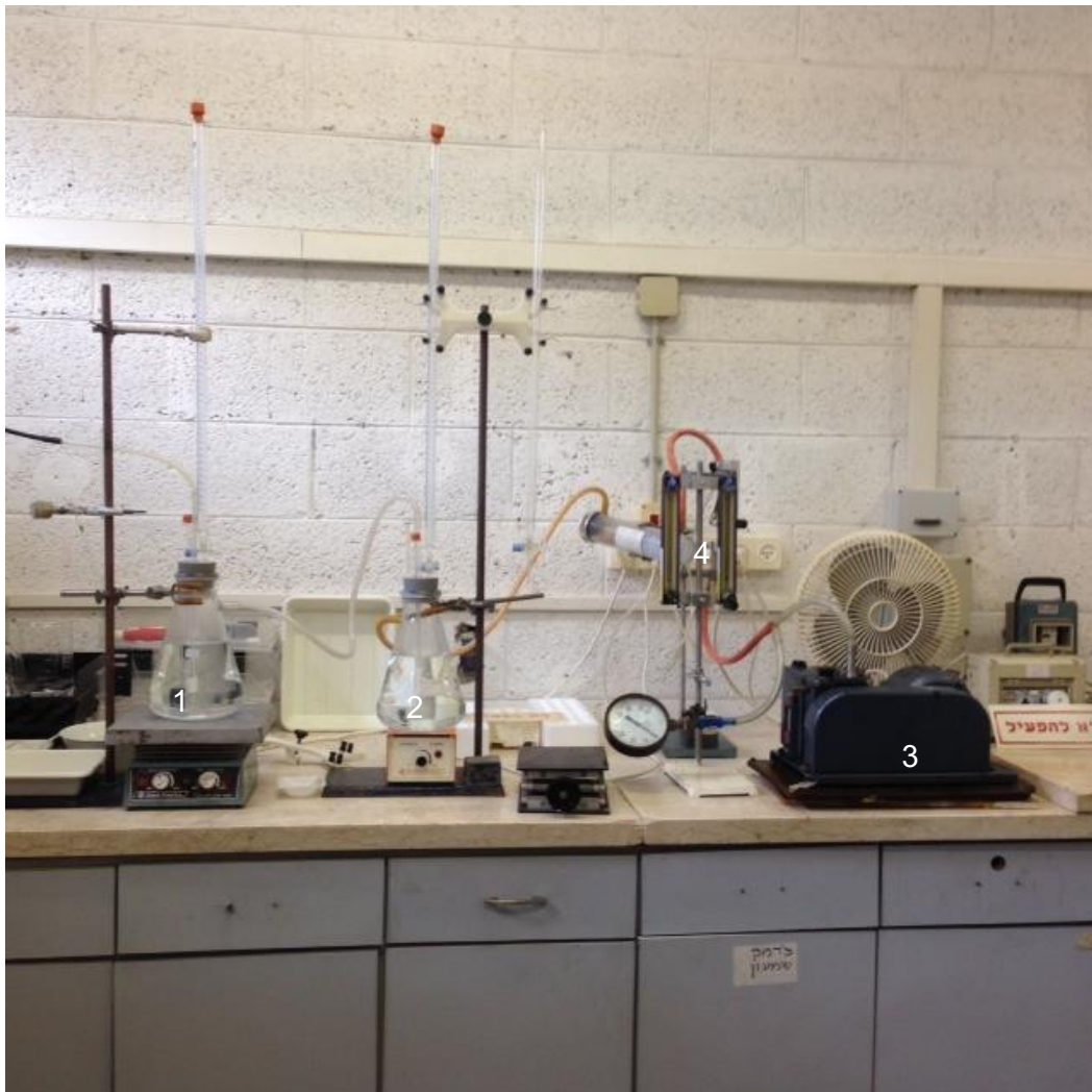
Figure 3: Pumping system and traps: (1) (2) traps through which air containing ammonia is passed, (3) pump which draws air through the system, (4) flow meter and valve to control air velocity
