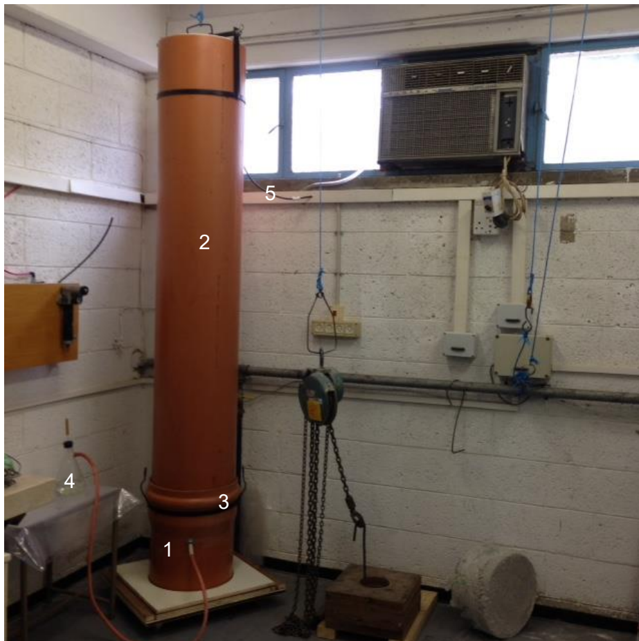
Figure 1: Testing system for monitoring ammonia emission from concrete; (1) concrete chamber (see Figure 2), (2) pipe into which ammonia is emitted and monitored, (3) connection between concrete chamber and pipe using an O ring, (4) air inlet and bubbling through water, (5) connection to pumping system (see Figure 3)
