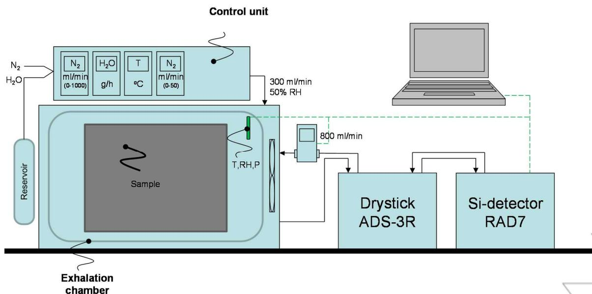
Figure 2 Schematic view of the thoron test facility.
